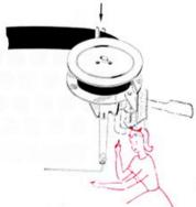
You can also use a bicolor ribbon, for instance black/red. Insert the ribbon in such a way that the black part will be on top. With the ribbon adjuster you will be able to obtain three settings:
