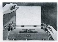
To remove the paper when you are finished writing, simply pull it up and out of the machine. If you wish, you can turn the cylinder knob at the same time to move the paper up. Some users prefer to pull the paper release forward, thus lifting the paper bail slightly.
