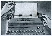
You are now ready to insert your sheet of paper. Drop the paper lightly behind the cylinder and turn the cylinder knob to bring it around and up until the paper shows in front of the cylinder.
