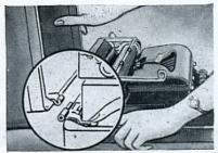
Unlock and throw open the top of the case. You can use your Royal Portable in the case if you wish. Simply press down the small lever and remove the top of the case by sliding it out to the right.
