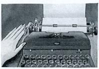
To return the carriage for another line of writing, push the carriage return lever to the right. This also automatically turns the paper to the next line when the carriage is returned. If you want to double-space instead of single-space, or to write on ruled lines, see instructions inside.
