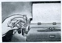
To set the margin, hold the MAGIC\* Margin lever forward and move the carriage so that the little arrow below the point where the type strikes is exactly where you want your left margin. (If you are moving the carriage to the left, press carriage release lever simultaneously.)
