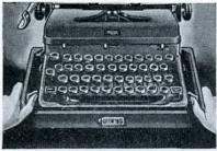
If you prefer to remove your Royal Portable completely from the case, press the two clip handles in the case on each side of the machine front and back, and then lift the machine right out of the case.
