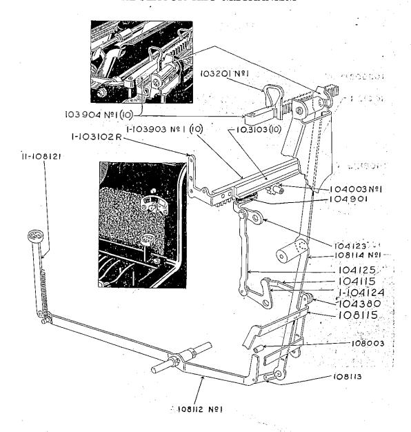
Rack assembly 1-103903 is disconnected from escapement gear 104003 by arm 104123, which is raised by the movement of the lower arm of vertical lever 108114 No. 1.
